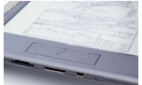
SD memory card slots in here as does USB PC connection
